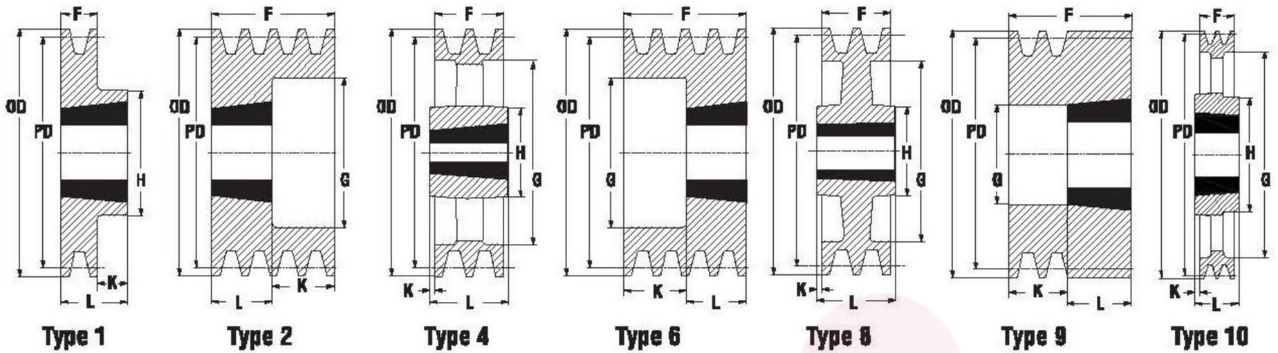
Dimensions for *Martin* pulleys are listed in the following tables with TB bushings in place. The type of pulley shown below is indicated by a number (1 to 11), and the construction is indicated by suffix number (-1 for solid, -2 for web and -3 for spoked).
